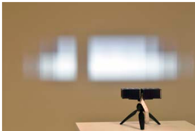
Segmented automotive LED high-beam unit realized as a micro-optical, irregular fly's eye condenser. The deactivated segment prevents glare from blinding oncoming traffic. © Fraunhofer IOF
