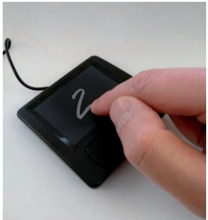
AIfES demonstrator for handwriting recognition. Numbers written by hand on the PS/2 touchpad are identified and output by the microcontroller. © Fraunhofer IMS
