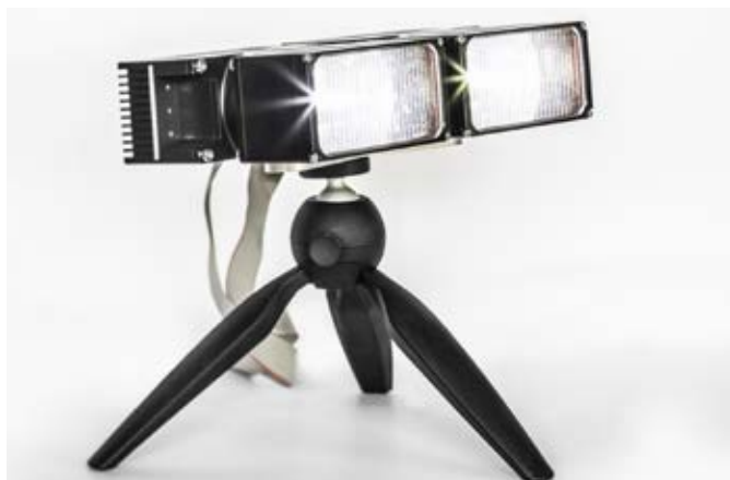
Segmented automotive LED high-beam unit realized as a micro-optical, irregular fly's eye condenser. Two identical modules assembled with 1.5° rotation to one another. © Fraunhofer IOF
