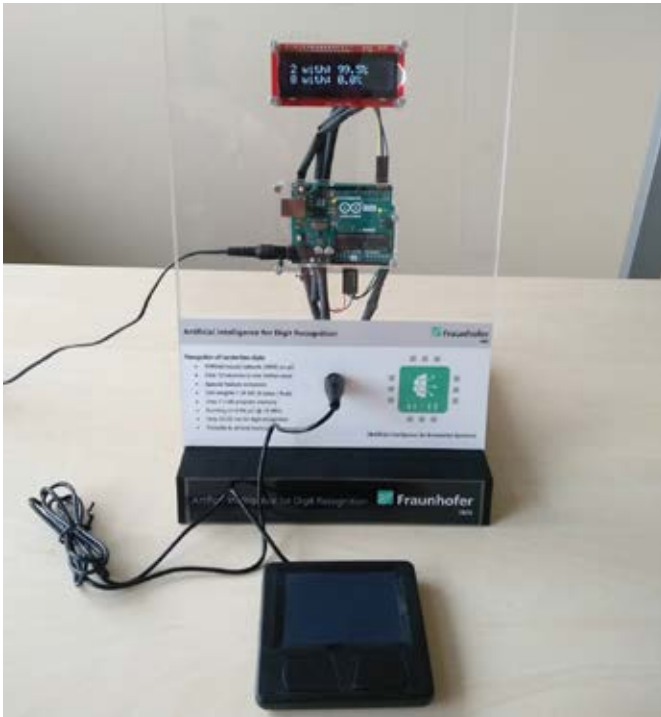
AIFES demonstrator for handwriting recognition. All functions have been integrated on the Arduino UNO, which reads the sensor values of the touchpad, performs number recognition and outputs the result to the display. © Fraunhofer IMS
