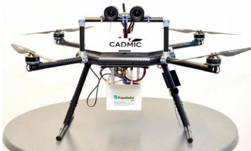
Drone with stereo camera. The small white box holds the embedded system, which evaluates the slightly offset images from the two cameras in real time in order to detect obstacles. © Fraunhofer IOSB
